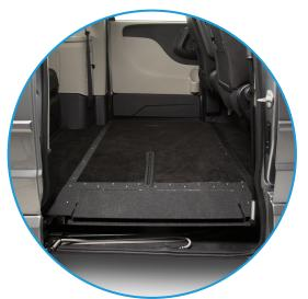
Stowed ramp is protected within the vehicle floor with no squeaking or rattling. In-floor ramp keeps dirt and debris from entering the vehicle cabin.
